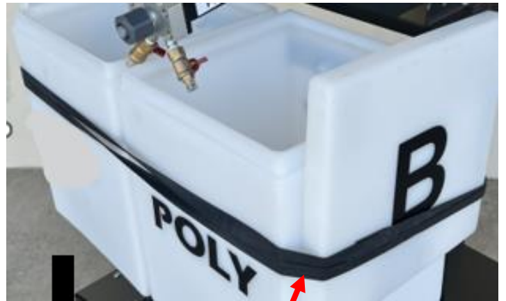
Holds lids to tanks when in use
